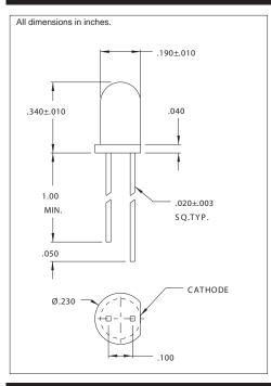
These LED lamps offer a variety of diffused lens effects and color availability. These lamps are available with both wide view angles and narrow view angles for high bright direct viewing. The High Efficiency Red and Yellow lamps are produced with GaAsP/GaP and the High Efficiency Green lamp is produced with GaP/GaP. This compact, rugged and lightweight LED lamp requires low power and allows for versatile PC board or panel mounting.
